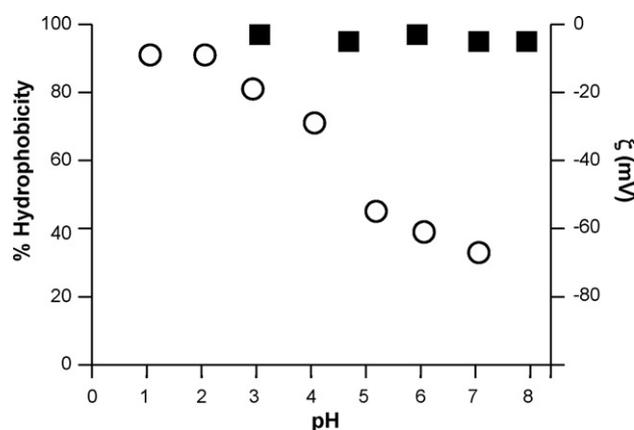
**Fig. 4.** Electro kinetics and hydrophobicity of *B. subtilis* PY79 spores. Zeta potential measurements of purified suspensions of PY79 spores ( $\circ$ ) in water between pH 1 and 12. Hydrophobicity of PY79 spores ( $\blacksquare$ ) determined by the SATH assay in the pH range of 3–8.
